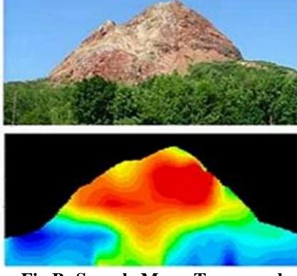
Fig B: Sample Muon Tomography Image
