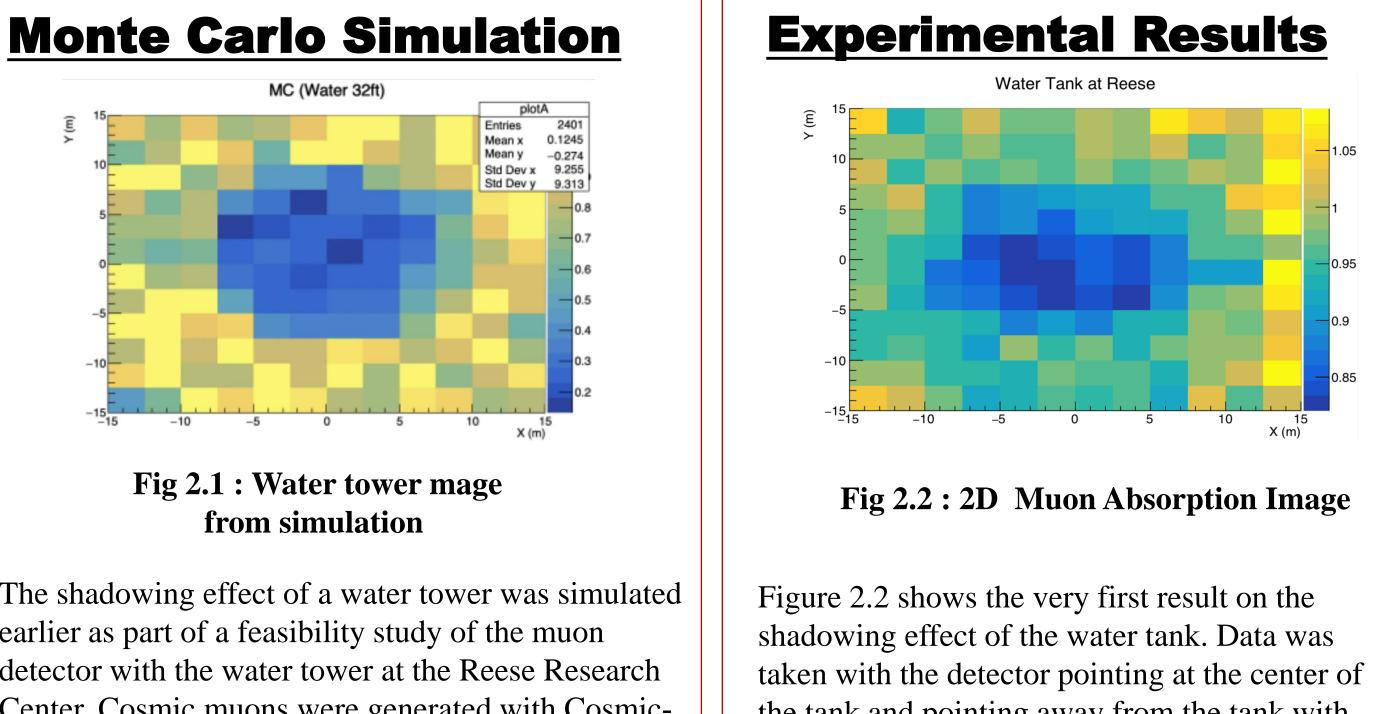
The shadowing effect of a water tower was simulated earlier as part of a feasibility study of the muon detector with the water tower at the Reese Research Center. Cosmic muons were generated with Cosmic-Ray Shower library (CRY) and propagated through a simplified water tank using Geant4. Muon tracks were reconstructed from hits in four trays each containing 11 scintillator bars.
