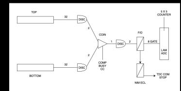
Fig 2. DAQ Trigger Process.
