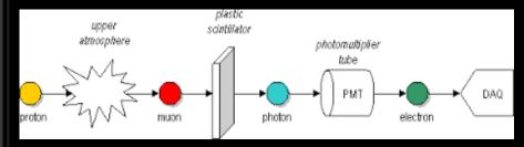
Fig 1. Schematic summarizing the muon detection process
